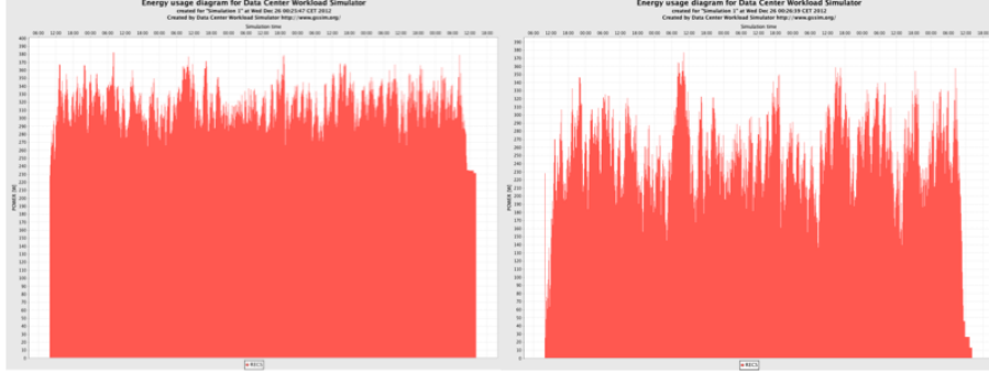
Figure 6: Comparison of energy usage for Random (left) and Random + switching off unused nodes strategy (right)
