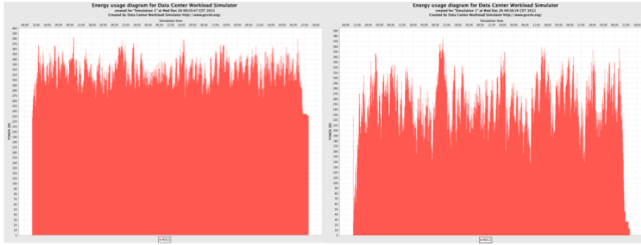
Figure 6: Comparison of energy usage for Random (left) and Random + switching off unused nodes strategy (right)
