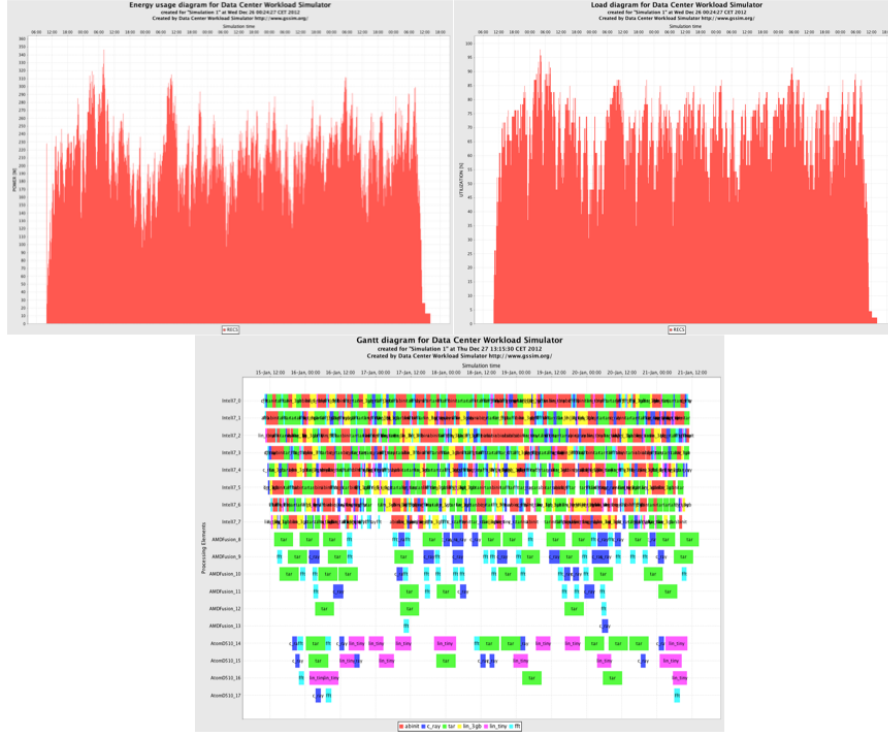
Figure 12: Energy usage optimization + switching off unused nodes strategy
