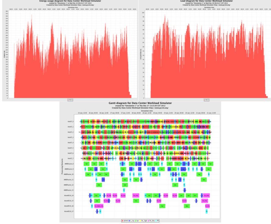
Figure 9: Energy usage optimization + switching off unused nodes strategy
